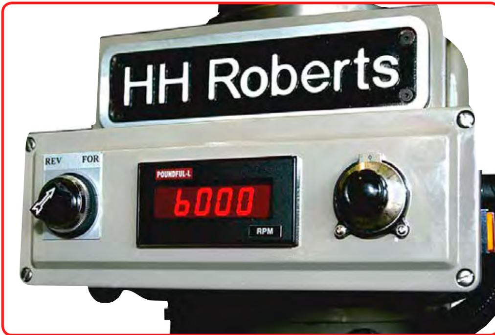
The controls are laid out to be instinctive for an experienced user. The forward / stop / reverse is on the left, The speed control is on the right. The speed knob is internally geared to allow easy setting of the speed. Speeds can be quickly and accurately set to within about 10 RPM.
