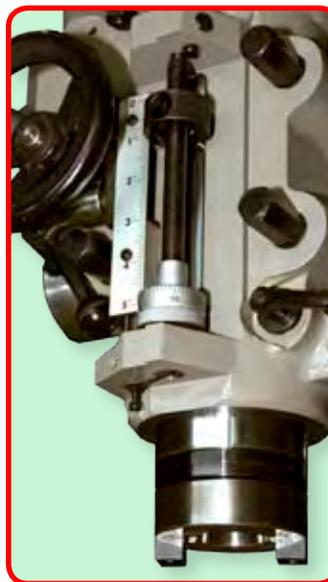
The optional # 40 taper spindle. # 30 and Erikson spindles can also be supplied.
