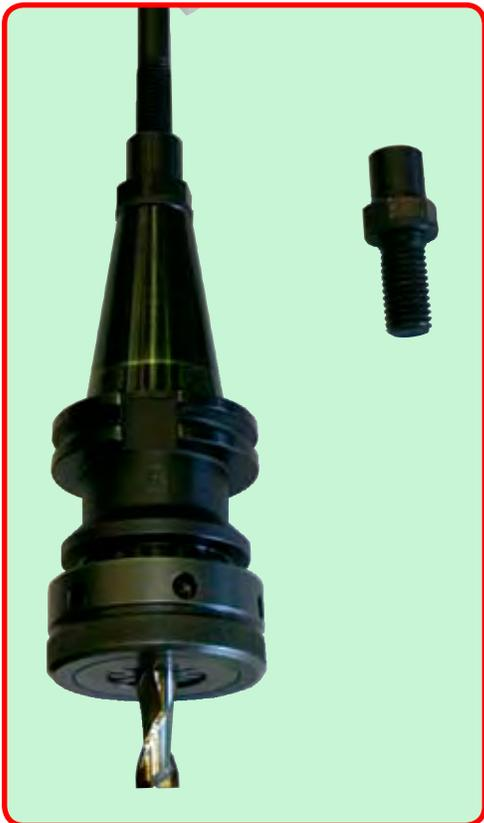
A typical Cat-V-40 collet chuck with the pull stud removed and our drawbar adapter and drawbar fitted. The adapter is shown separately to the right.
