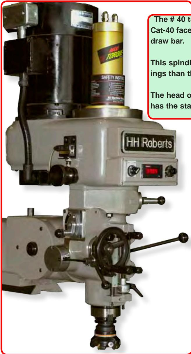
The # 40 taper spindle with a Cat-40 face mill and the power draw bar.
